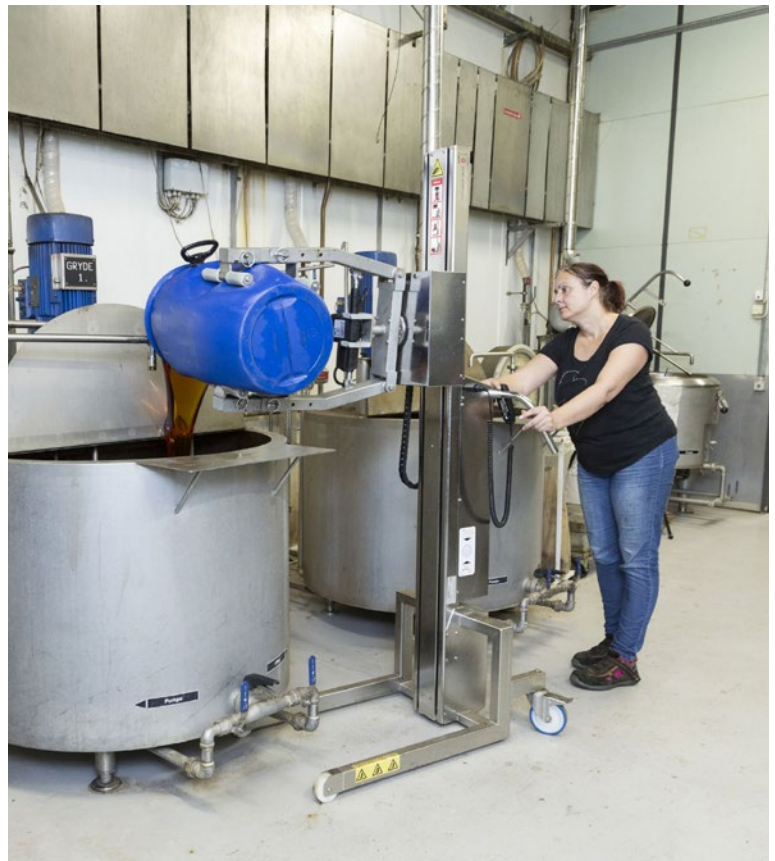
Drum turner 87924 with motorized grip and rotation
